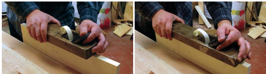
The long and the short of it. Most Japanese planes are about 10½" long (left). The naga-dai kanna , the Japanese equivalent of a try plane, is the exception to this rule, being about 15"-16" long (right).
