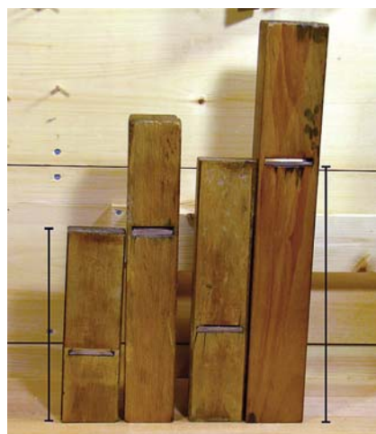
Separated at birth? When the reference lengths of the chū-shiko kanna and a fore plane are compared side by side, they are nearly identical in length. The same is true for a naga-dai kanna and a try plane.
